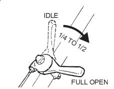
Figure 7. Throttle Lever (1/4 to 1/2)
